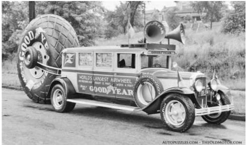
In 1929, the Goodyear Tire and Rubber Company introduced its first Airwheel, a low-pressure balloon tire for use on airplanes. Alvin J. Musselman developed this tire that Goodyear referred to as the Musselman type in its press releases. It used a small rim and a large section tire that was capable for carrying heavy loads. În airplane use, it also eliminated the need for costly shock absorbers due to it's cushioning abilities.
