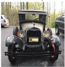
When I started to bring the car to cruise nights at Lapp's I started seeing the temperature creep up. The more I flushed it the worse it got. I couldn't go five miles without boiling over. I finally took the radiator to Penns Grove to be repaired. When they got the top off and rodded it out it appeared that at some time the radiator cap was left off and a mouse built a nest in there.
