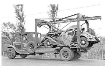
One look at this truck with a wrecked mid-1930s coupe on board told us that this wasn't your run of the mill International tow truck used for bringing in inoperable or crashed cars. After some thought, it appears that this machine may have been an old rigger's truck pressed into service by Andrew Murphy & Sons of Omaha, NB, for picking up and transporting damaged cars.
